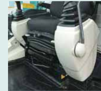
Seat suspension absorbs vibration
