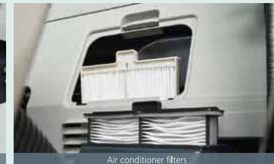
Air conditioner filters
