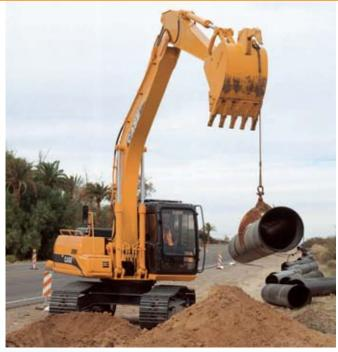
The standard Power Boost and Auto Work Mode on the CX130 and CX160 optimize productivity on any job site. And like all CX models, these machines offer a choice of three optional auxiliary hydraulics packages to meet your application needs: single-acting one pump, double-acting single or dual pump, and double-acting general purpose for use with the optional thumb kit.
