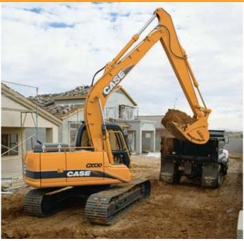
Like all CX excavators, two-pump flow on boom/arm circuits assist boom lowering and arm closing speed to trim work cycles. And features like free swing control help keep loads moving quickly and efficiently.
