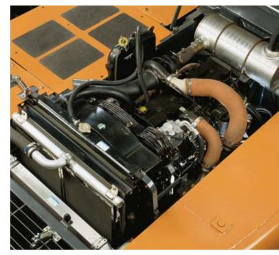
The 24-valve cylinder head in the Case engine features centered fuel injection, which improves combustion and produces 20 percent better low-end torque and response. Electronic injection supplies higher injection pressure for better fuel atomization, resulting in a cleaner burn, superior fuel economy, and outstanding engine performance.
